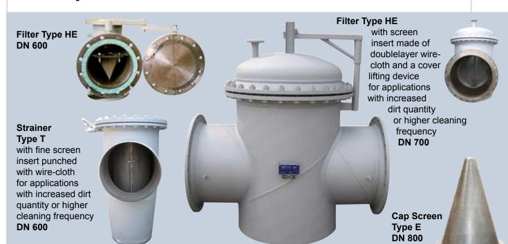
Protective strainers are applied in the pipeline construction in front of pumps, compressors or control vales. Depending on the process, particles will be filtered out from water, condensate or gas, in order to protect the plant components from damage.
